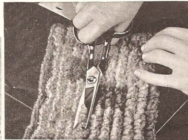
Shearing off the ends of the yarn to give a smooth pile effect
